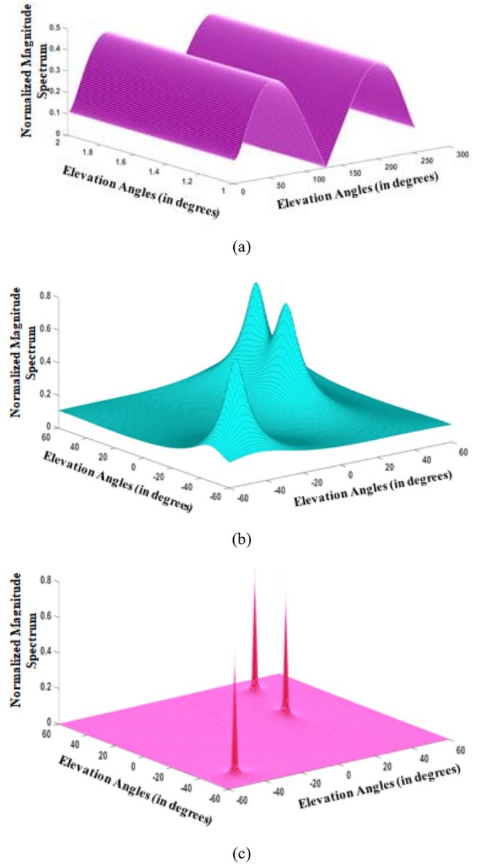
Fig. 5 Variation of normalized magnitude of DoAs at the frequency of 10 GHz using the hybrid antenna array consistent with Fig. 1, and (a) without performing any optimization method, (b) with performing the LS-SVM optimization method with three classes, and (c) with performing the DNN-RBF optimization method with the 5 hidden layers and 49 neurons and three classes
