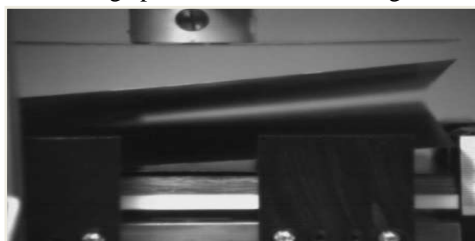
Fig. 7 Wafer lifting during picking process
