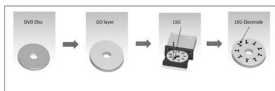
Fig. 1 The overall process of patterning LSG electrodes
