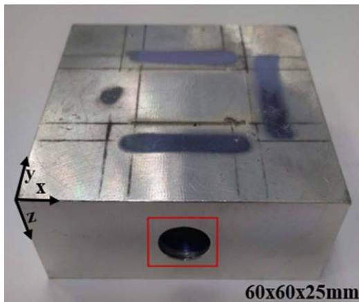
Fig. 1 Sample representing the 10 mm diameter hole
