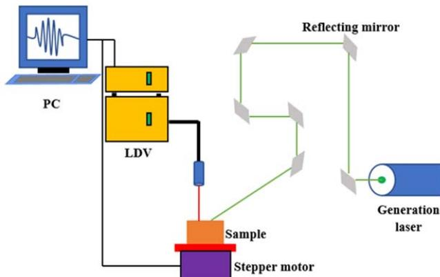
Fig. 4 Schematic representation of the experimental setup
