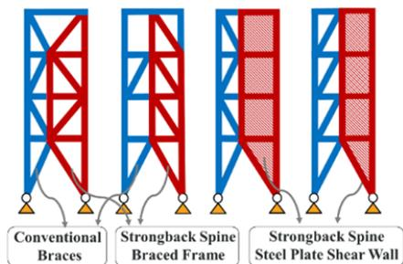
Fig. 2 Different SBS configurations
