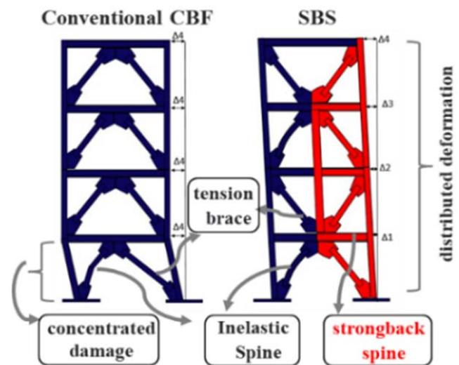
Fig. 1 The effect of strongback spine on distribution of displacement throughout the structure
