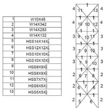
Fig. 4 Detail member sections of the SBS
