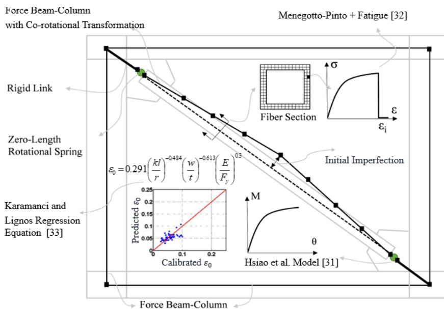
Fig. 5 Nonlinear modeling details used in this study
