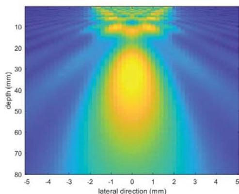
Fig. 6 Ultrasound field corresponding to the rectangular element
