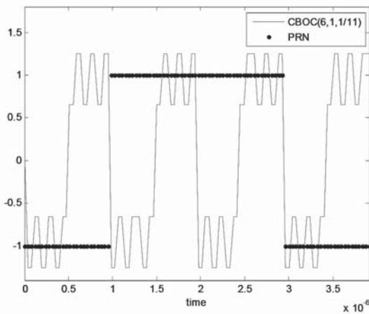
Fig. 2 CBOC(6, 1, 1/11) signal with length of 4 chips
