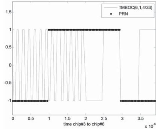
Fig. 3 TmBOC(6, 1, 4/33) signal with length of 4 chips
