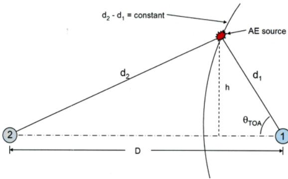
Fig. 5 D location on an infinite plate [2]
