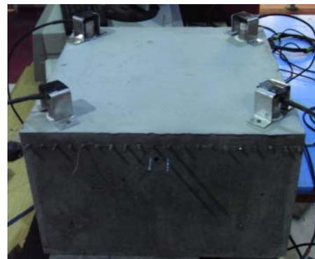
Fig. 9 Photograph of specimen with sensors setup
