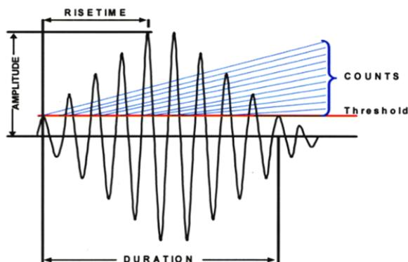
Fig. 3 Characteristics of a burst type of AE signal [8]
