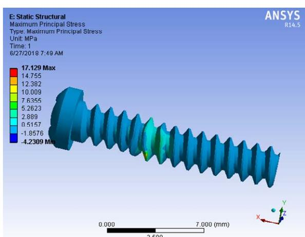
Fig. 6 (e) Maximum principal stress in critical screw
