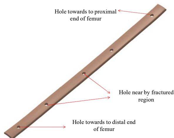
Fig. 3 Customized implant designed for fractured bone
