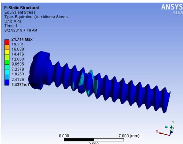
Fig. 5 (e) Von-Mises stress distribution in critical screw
