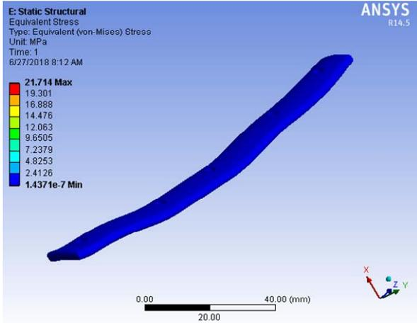
Fig. 5 (c) Von-Mises stress distribution in implant
