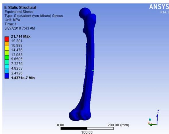
Fig. 5 (a) Von-Mises stress distribution in clinical setup
