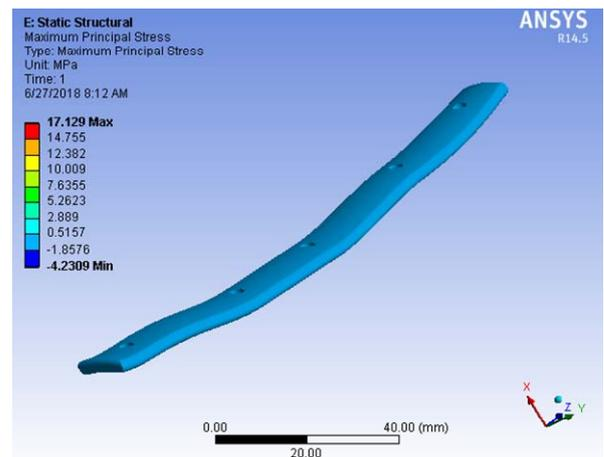
Fig. 6 (c) Maximum principal stress in implant
