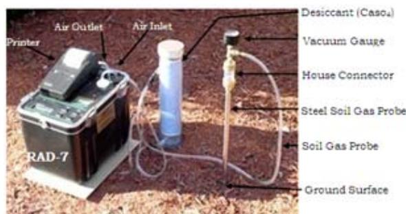
Fig. 3 Setup of the Radon-222 measurement equipment
