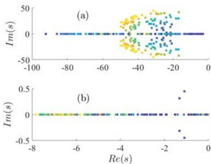
Fig. 6 Pole maps, on the  $y$ -axis is the imaginary part of the pole,  $Im(s)$ , and the  $x$ -axis is the real part of the pole,  $Re(s)$ : (a) Pole map of the inner closed-loop system, (b) Pole map of the outer closed-loop system. The color code indicates the level of  $\|k\|_F$ , where red denotes the highest value, and dark blue denotes the smallest
