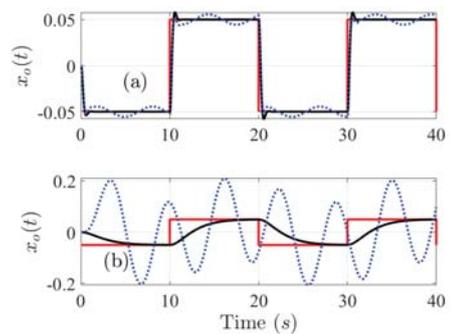
Fig. 9 Ball position versus time. (a) Controlled system response at  $\min(F_1)$ , (b) Controlled system response at  $\max(F_1)$ . Red solid line: reference signal  $x_d(t)$ , black solid line: system response with  $d_i(t) = d_o(t) = 0$ , blue dotted line: system response with  $d_i(t) = d_o(t) = 0.5\sin(t)$
