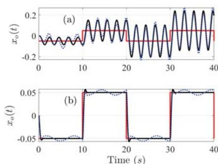
Fig. 10 Ball position versus time. (a) Controlled system response at  $\min(\|k\|_F)$ , (b) Controlled system response at  $\max(\|k\|_F)$ . Red solid line: reference signal  $x_d(t)$ , black solid line: system response with  $d_i(t) = d_o(t) = 0$ , blue dotted line: system response with  $d_i(t) = d_o(t) = 0.5\sin(t)$
