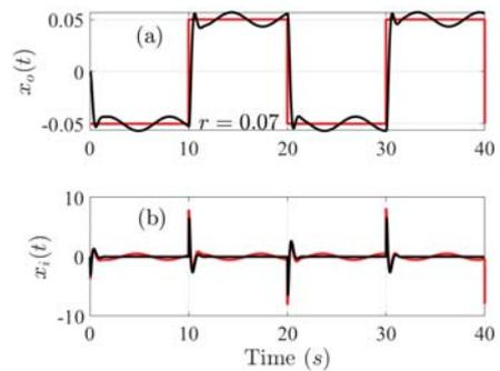
Fig. 8 Outer and inner controlled systems' responses when  $r = 0.07$  (a) Response of the outer closed-loop system  $x_o(t)$  versus time, (b) Response of the inner closed-loop system  $x_o(t)$  versus time. Red solid line: reference signal, Black solid line: actual system, response response with  $d_i(t) = d_o(t) = 0.5\sin(t)$
