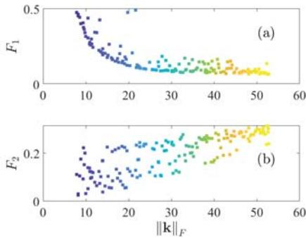
Fig. 4 Projections of the Pareto front: (a)  $F_1$  versus  $\|k\|_F$ , (b)  $F_2$  versus  $\|k\|_F$ . The color code indicates the level of  $\|k\|_F$ , where red denotes the highest value, and dark blue denotes the smallest.
