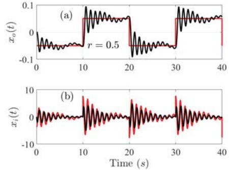
Fig. 7 Outer and inner controlled systems' responses when  $r = 0.5$  (a) Response of the outer closed-loop system  $x_o(t)$  versus time, (b) Response of the inner closed-loop system  $x_o(t)$  versus time. Red solid line: reference signal, Black solid line: actual system, response response with  $d_i(t) = d_o(t) = 0.5\sin(t)$
