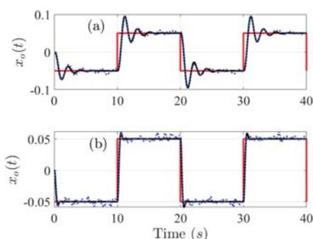
Fig. 11 Ball position versus time. (a) Controlled system response at  $\min(F_2)$ , (b) Controlled system response at  $\max(F_2)$ . Red solid line: reference signal  $x_d(t)$ , black solid line: system response with  $n_i(t) = n_o(t) = 0$ , blue dotted line: system response with  $n_i(t) = n_o(t) = WN$
