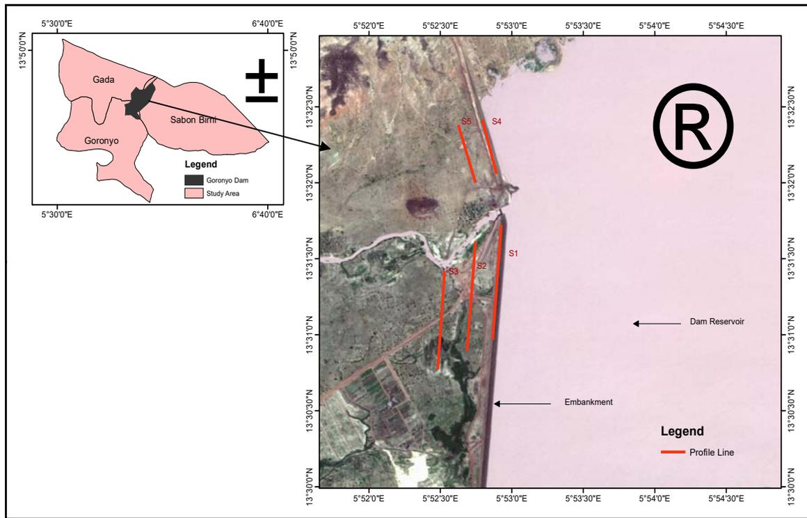
Fig. 2 Field Survey Layout Using Wenner Electrode Configuration
