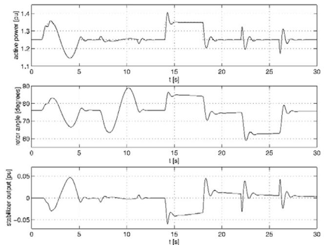
Fig. 6 Generator active power  $P_e$ , rotor angle  $\delta$  and stabilizer output  $u_p$  for weak damped conditions in operating point  $P = 1.25$  [pu],  $\cos \varphi = 0.95$  with direct adaptive control power system stabilizer
