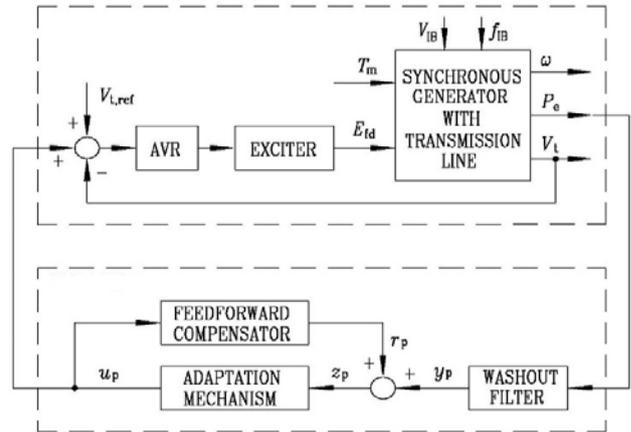
Fig. 2 Block diagram of the direct adaptive control power system stabilizer
