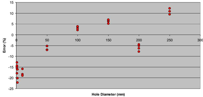
Fig. 11 Error in Stress-Intensity Factor Using Absolute Weighting Function
