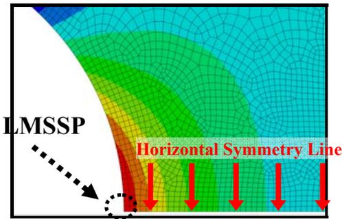
Fig. 5 LMSSP for Flat Plate with Circular Hole
