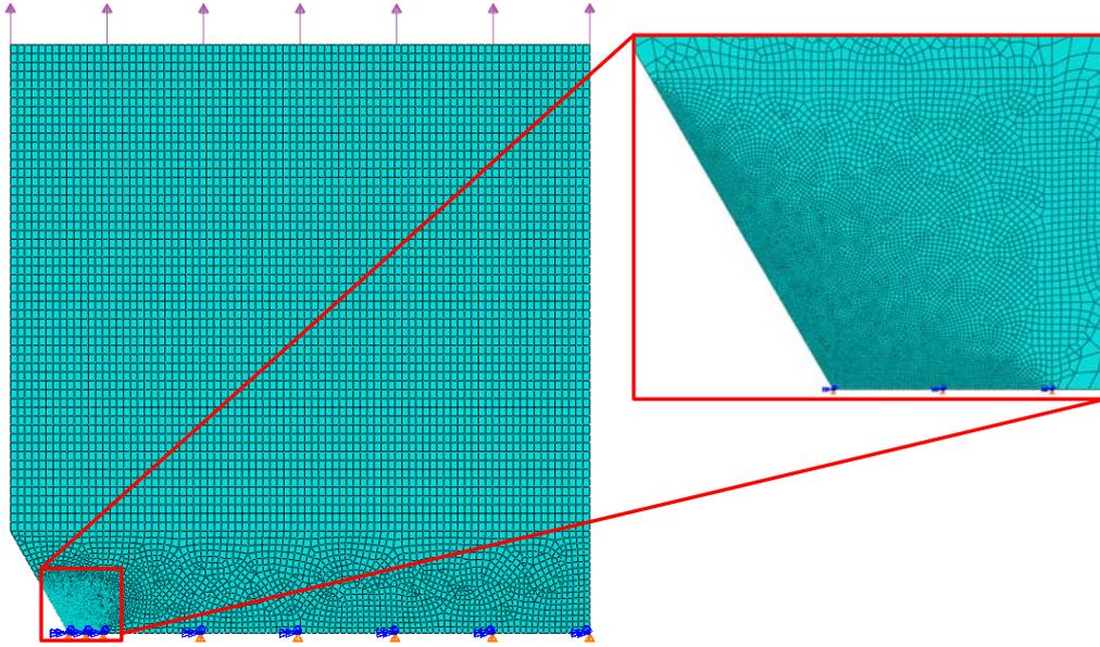
Fig. 13 Half-Symmetry Model for 120-Degree V-Notch Case
