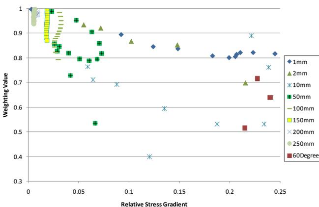
Fig. 20 Absolute Weighting Function Values for Notch
