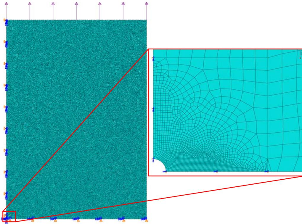
Fig. 4 Quarter Symmetry Model for 1-mm Hole Case
