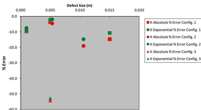
Fig. 18 Stress-Intensity Factor % Error for All Configurations-Thick Cylinder
