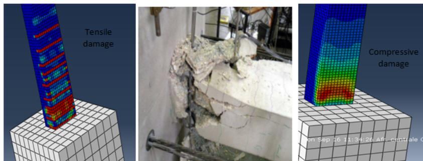
Fig. 6 Comparison of the local failure
