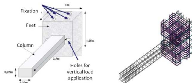
Fig. 1 Geometry and reinforcement of the sample used in the present study
