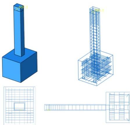
Fig. 3 Finite element idealization (Geometry and reinforcement)
