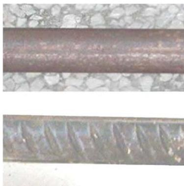
Fig. 3 Bars used as reinforcement [16]
