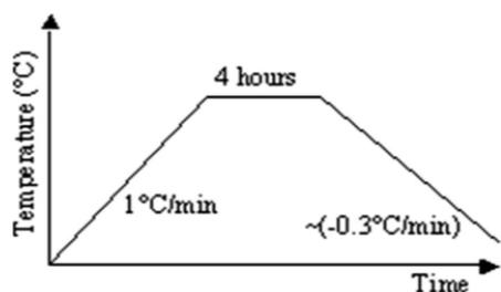
Fig. 7 Thermal degradation of concrete models [18]
