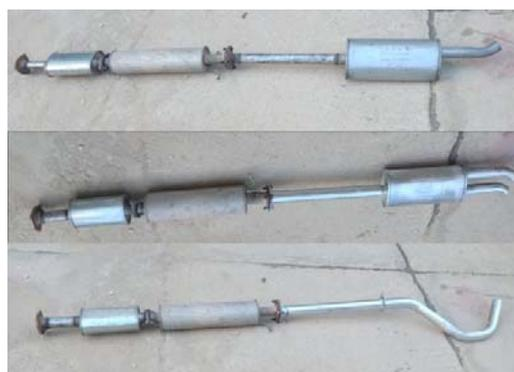
Fig. 2 Construction of the expansion chambers
