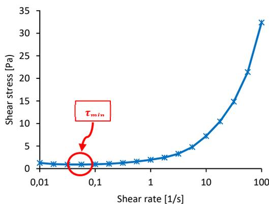
Fig. 3 Identification of the yield stress of cement paste for w/c = 0.5 and PC = 0.12%
