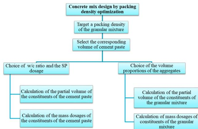
Fig. 1 Concrete mix design methodology
