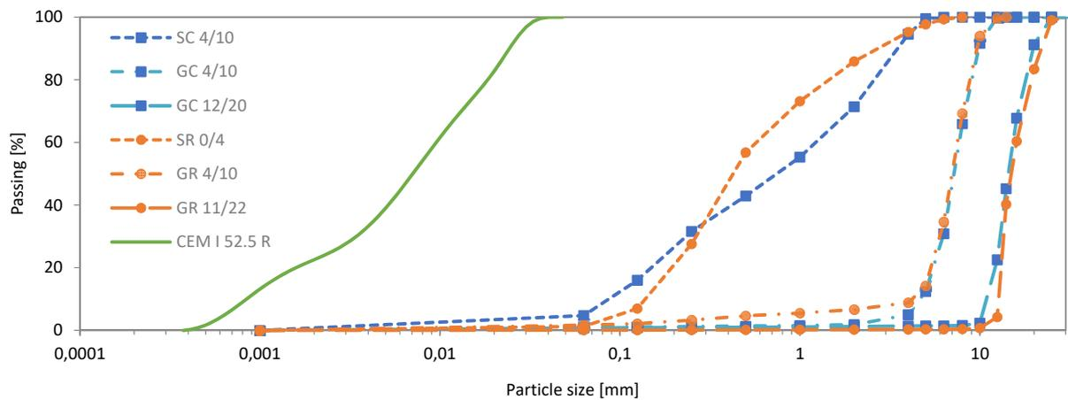
Fig. 2 Particle size distribution of the materials of the study
