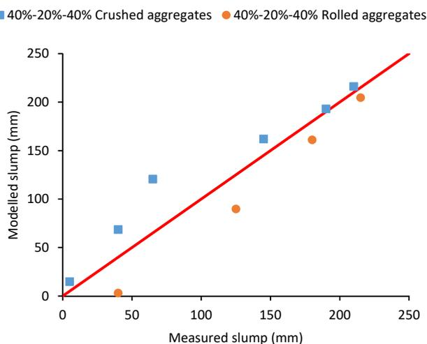
Fig. 7 Measured slump vs. modelled slump
