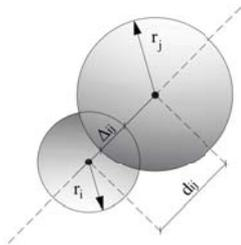
Fig. 2 The contact model between two particles
