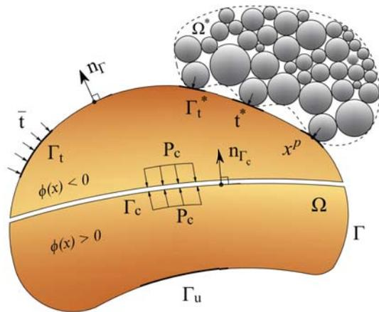
Fig. 1 The interaction of in-contact continua with discontinuum
